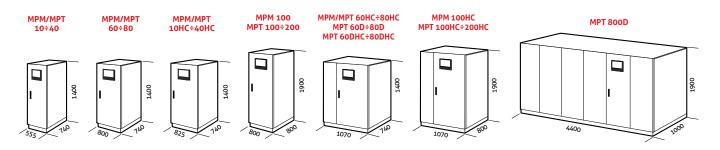
HC= Version with filtering of 5<sup>th</sup> or 11<sup>th</sup> harmonics D= Twelve-phase version
